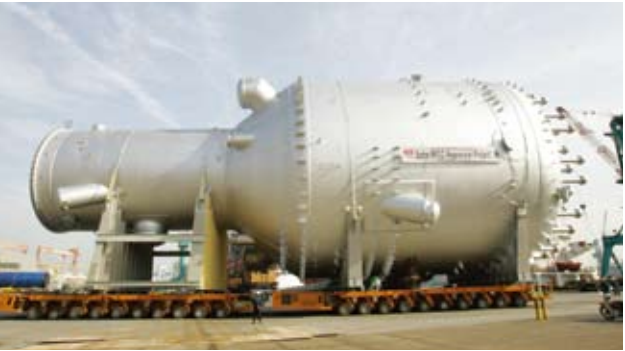
RFCC reactor shipment In August, we shipped a residue fluidized catalytic cracking (RFCC) reactor ordered by GS Engineering & Construction for the Ruwais Refinery expansion project in the United Arab Emirates. The reactor is the largest unit of its kind in the industry at 46 meters in height, 14 meters in circumference, and 1,150 tons in weight. RFCC reactors play a key role in the refining process, converting low-quality crude oil into value-added fuel products.
